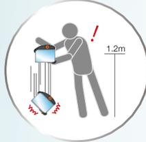
\*) Drop resistance has been tested for tablet weights up to 1.1 kilogram.
