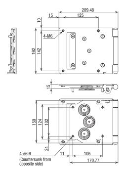
Includes 4 screws (M6x16 hexagon socket countersunk screw) for mounting on the main unit of the Assist Wheel Drive.
